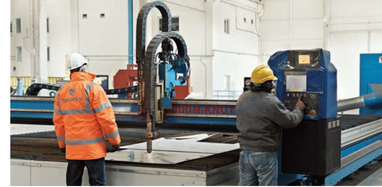
Cutting capacity of up to 60 mm with CNC plasma and up to 200 mm with oxygen
