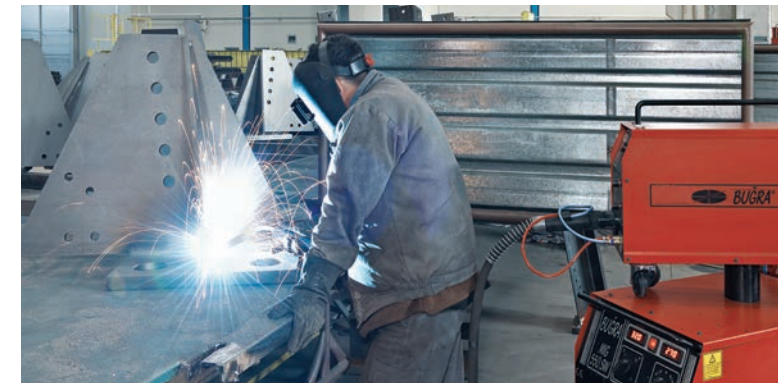
Gas metal welding machines (550 Amp)
