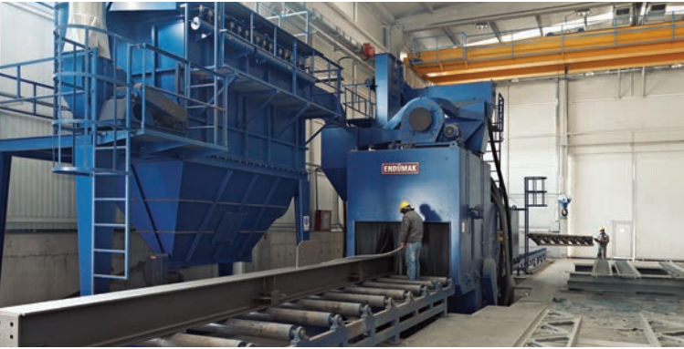
Up to 100 tons/daily - Sandblasting and surface preparation with Sa 3 quality
