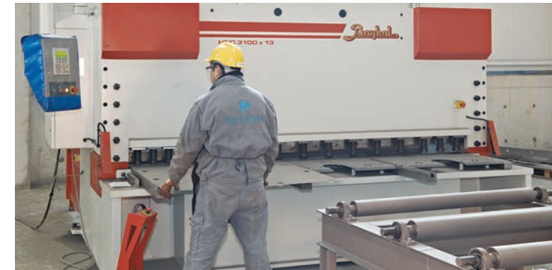
Blanking capacity of up to 13 mm in thickness and 3,000 mm in width
