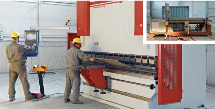
Plate bending capacity of up to 16 mm in thickness and 3,000 mm in width and plate bending up to 25 mm with a hydraulic cylinder.
