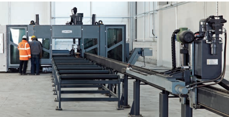
3-dimensional fully Computer Numerically Controlled (CNC) perforating and stamping
